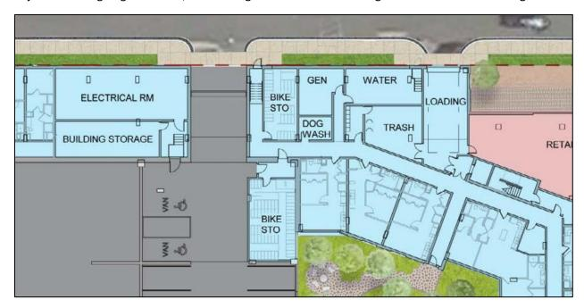
Staff wants to ensure minimal obstructions to bicyclists when entering and exiting the storage area. Staff recommends the doors leading to the bike room be automatic to allow ease of access to individuals bringing their bikes indoors. The bike storage area should also include a wall mount bike pump and bike repair stand.
