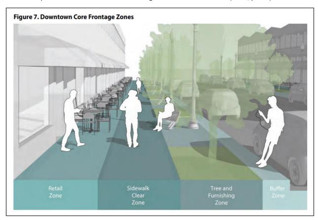
On America Boulevard, a build-to line of 15' is proposed with the applicant requesting a modification to provide less than the 20' frontage zone provided by the TDDP. The proposed frontage zone will include a 6' clear sidewalk zone, 4' tree and furnishing zone, and 5' buffer zone.
