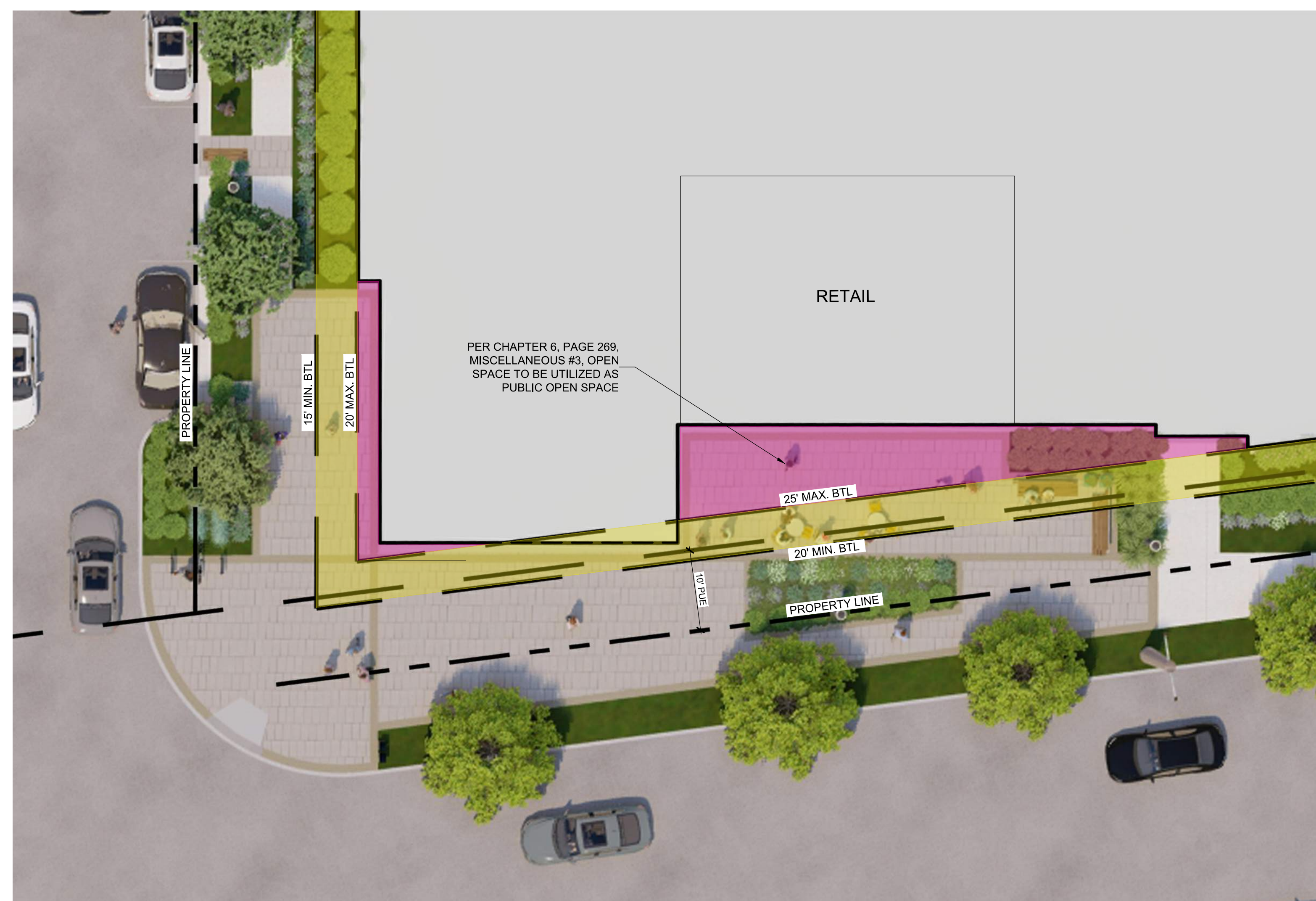
2 ENLARGEMENT - STREET FRONTAGE / FACADE WITHIN BUILD-TO-LINE L1-08 1"= 10'
