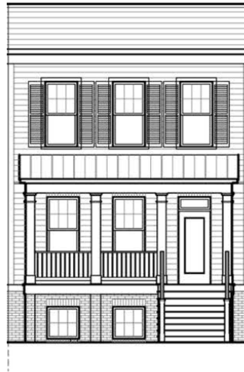
FRONT ELEVATION (one level porch)
