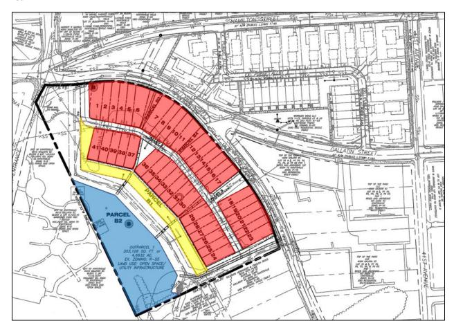
The site plan also includes an alley within the interior of the site, to provide services and site access, along the rear of the proposed units.
